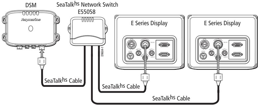
Configuring an E Series System - Multiple Displays
