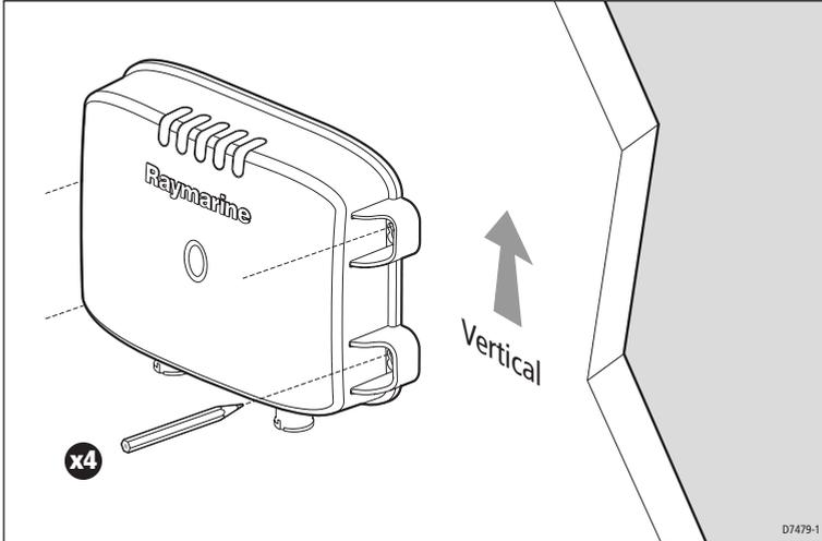
3. Drill a 9/64" pilot hole at each of the marked locations.
