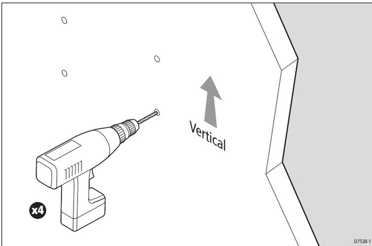
**Note:** For fiberglass with a gelcoat surface, you should overdrill the surface to prevent the gelcoat from chipping when driving in the screw. Before drilling the pilot hole, hand drill the marked location with an oversized bit and countersink to approximately 3/8" diameter.
