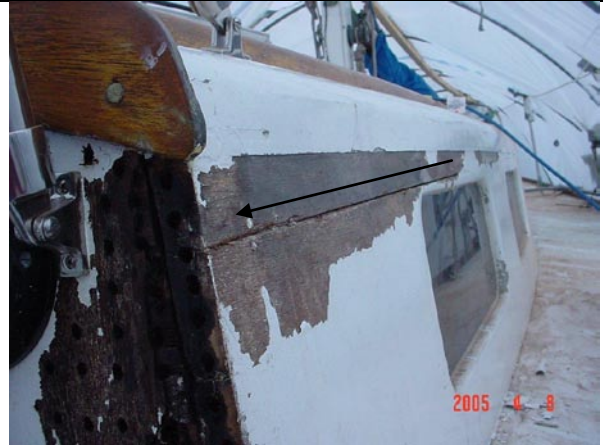
Coachroof joint that the water ran along to soak the bulkhead.
