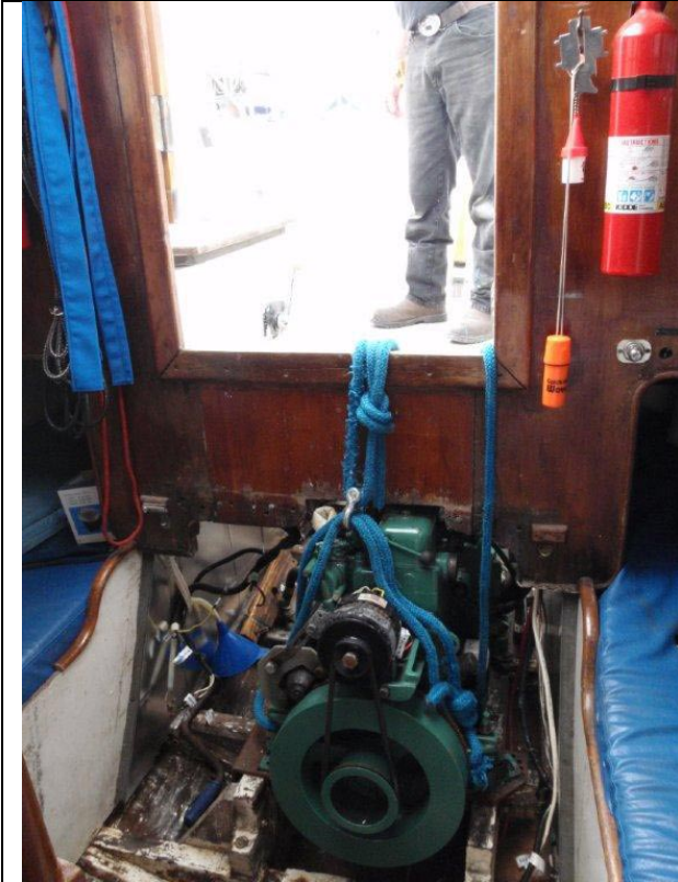
Old engine rigged for lifting
