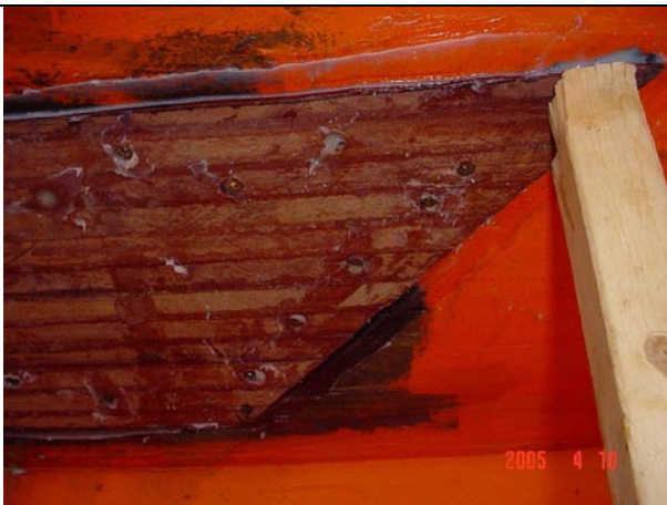
The finished hole with scarf joint all around
