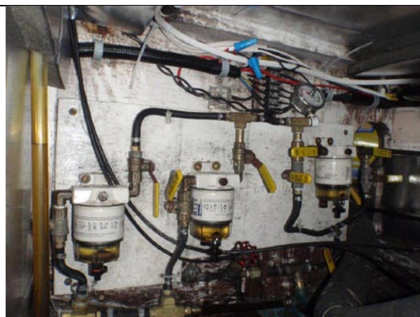
Filter bank mounted on the engine compartment aft bulkhead.
