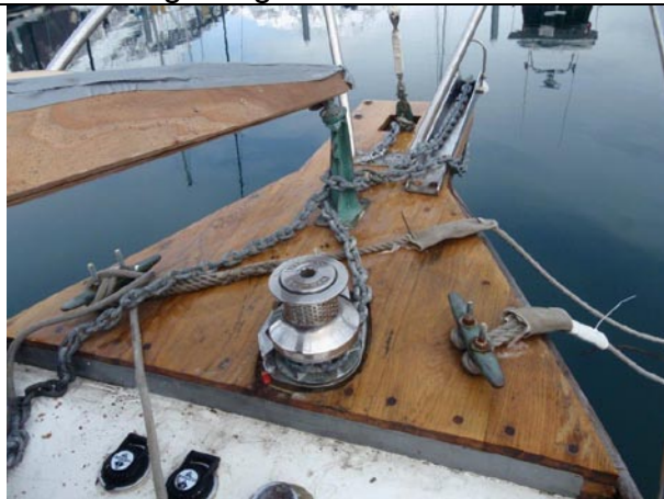
White oak apron with windlass hardware. In these photos, the anchor has been led back to the foredeck for the winter and multiple winter dock lines criss-cross the apron. In the sailing season the 35# Delta anchor rests in the Garhauer bow roller.
