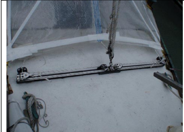
New Garhauer mainsheet traveler. You can also see the edge of the prototype cockpit cover.
