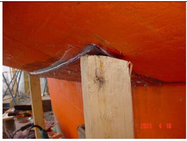
Mating dutchman with scarf joint all around
