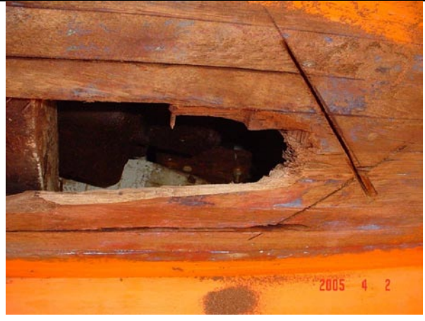
As the rot was removed the hole got bigger. Saw lines in solid wood are visible around the hole.
