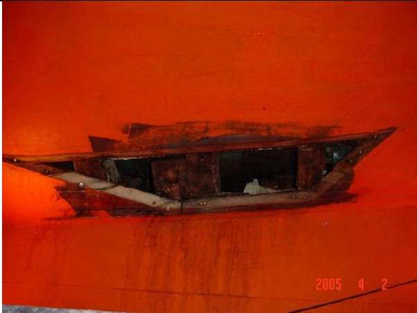
The finished hole with scarf joint all around
