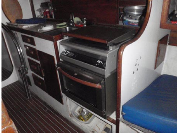
Galley Range with stovetop cover "down" for cabin heating.
