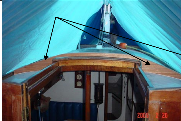
A custom yoke formed a bridge over the hatch for dodger mounting.
