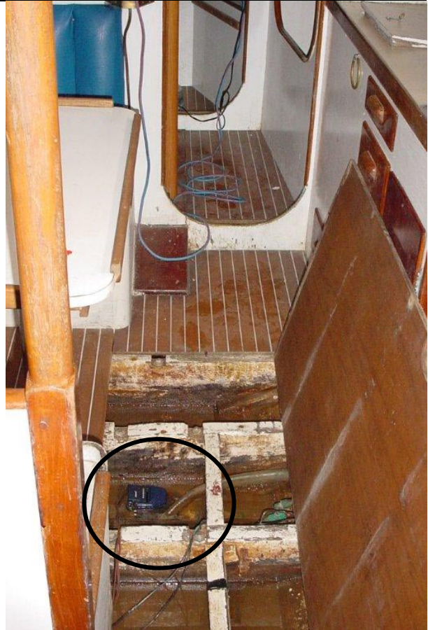
The old float switch allowed about an inch of water to stay in the bilge. It would switch off after water receded about ½ inch.
