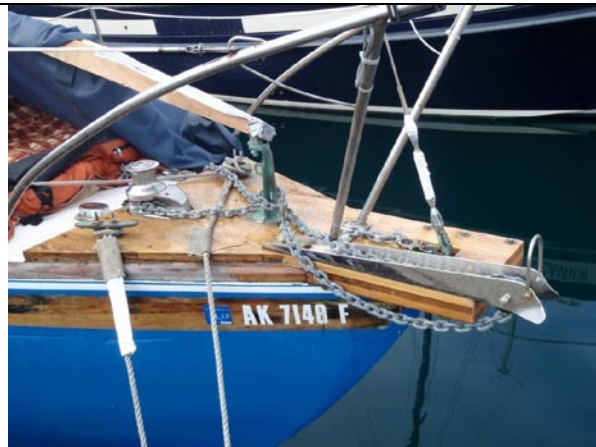
White oak apron with windlass hardware. In these photos, the anchor has been led back to the foredeck for the winter and multiple winter dock lines criss-cross the apron. In the sailing season the 35# Delta anchor rests in the Garhauer bow roller.
