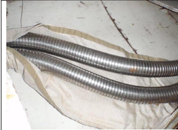
Galley range exhaust pipes led aft under the starboard quarterberth.
