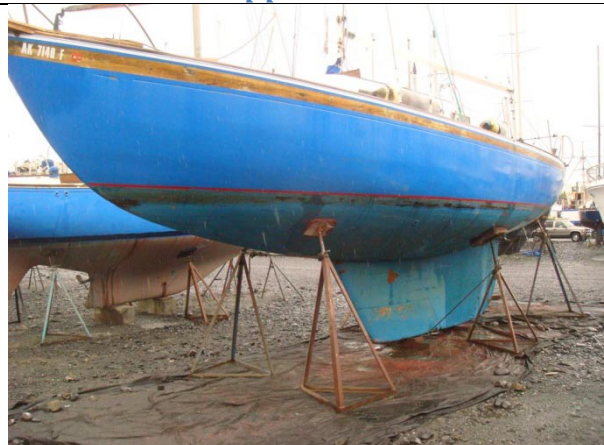
The hull refinishing project - stripped bare
