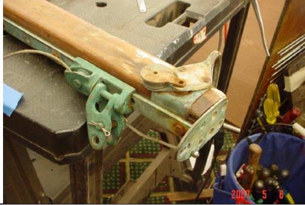
Iron bolts had corroded and stained the bronze fittings.
