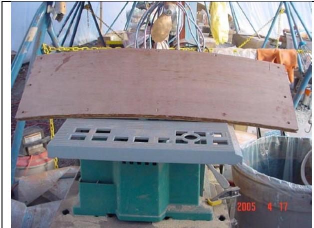
Laminated name board, pre-curved to fit transom.
