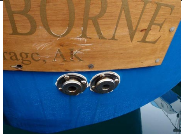
Galley range exhaust pipes terminate on transom. Burner fumes are removed from the cabin.
