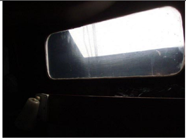
Cover had windows aligned with port lights so the cabin wouldn't seem like a cave.
