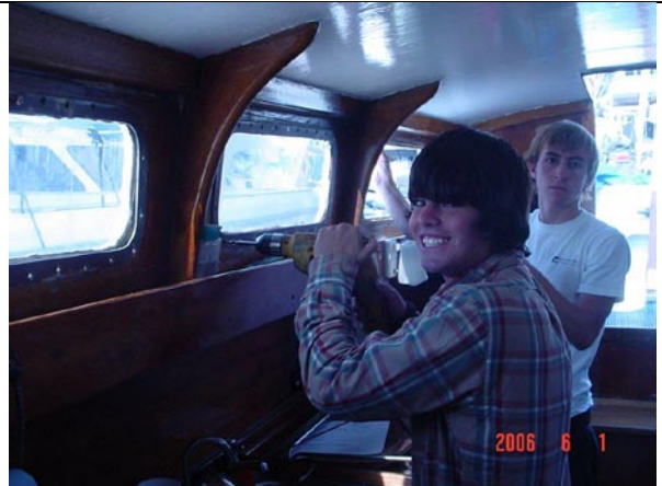
Spencer’s friend installing cleaned and prepped portlight
