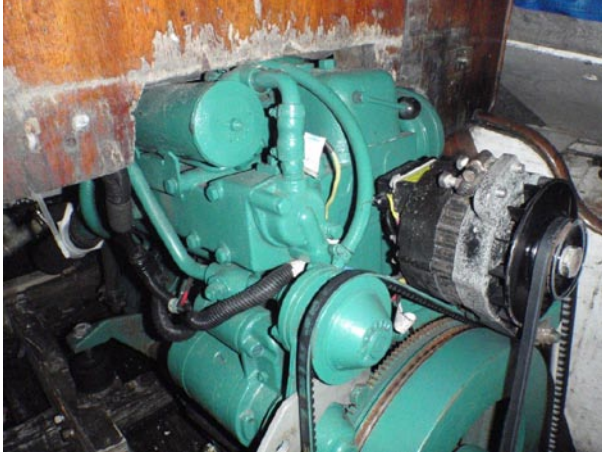
Water pump belt runs under the alternator. A custom mounting bracket was required to tension the alternator belt.
